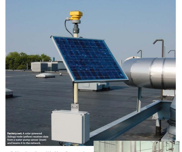
on all of the pods coordinates which of them talk to one another and when. The sensor nodes "listen" for one another and set up times to share data, while a network clock keeps the nodes in sync. The network resembles a mesh rather than the hub-andspoke arrangement used for cell phones; instead of linking each sensor directly to a central communication point, the nodes send data only to neighbors within radio range, saving power.
