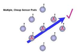
Figure 2. Multiple sensors provide lower resolution but more data and thus can yield sophisticated results.
