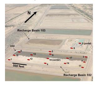
Figure 2: Oblique aerial photograph showing the location of the individual pods of the Sensor Web system at CAVSARP. The portal pod 0 is connected to a local server for Internet access.
