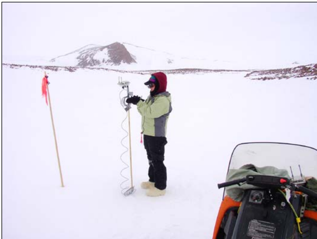
Figure 5: Sensor Web 3.0 deployment on East Antarctic Ice Sheet. Bamboo is used as the mounting stake for its known resilience to the harsh Antarctic conditions. Wires connect the pod to the temperature sensors at the surface. Note the second pod located in the snowmobile in lower right corner.
