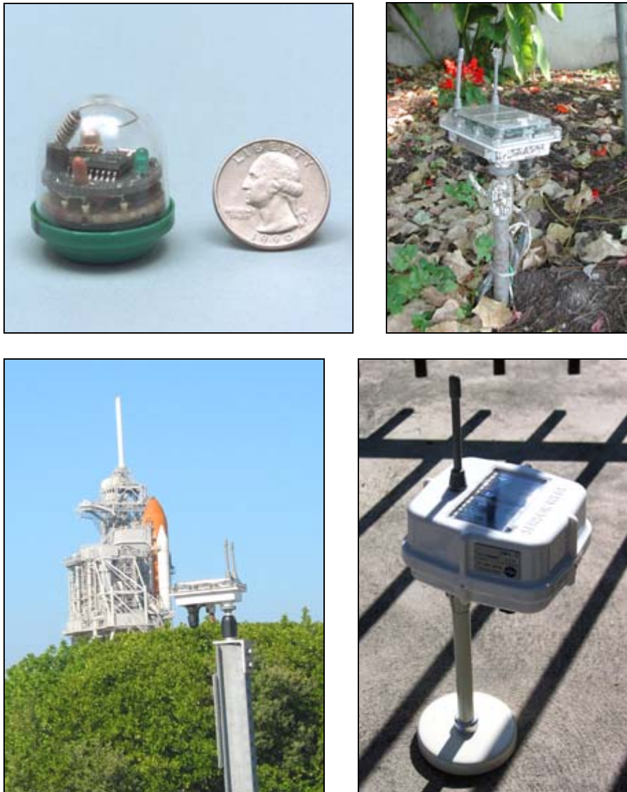
Figure 3: Various Sensor Web pods. Top Left: Functioning Sensor Web 1.0 pod, circa 1998. Note the small size which includes antenna, battery, and temperature and light sensors. Top Right: Sensor Web 3.1 pod deployed at the Huntington Botanical Gardens, circa 2002. It is about the size of two decks of playing cards. The pod is mud spattered from rain and watering and has a chewed antenna. Subterranean sensors (soil moisture and temperature) can be seen going into the ground. Bottom Left: Sensor Web 3.1 pod deployed less than a quarter mile from Space Shuttle Launch Pad 39A at NASA Kennedy Space Center (note shuttle on pad). This Sensor Web measured environmental conditions in the lagoons surrounding the launch site. Bottom Right: A Sensor Web 5.0 pod, circa 2004. This new generation of Sensor Web pods is more compact and more power efficient than previous ones, a direct result of exploiting Moore's Law in its design.
