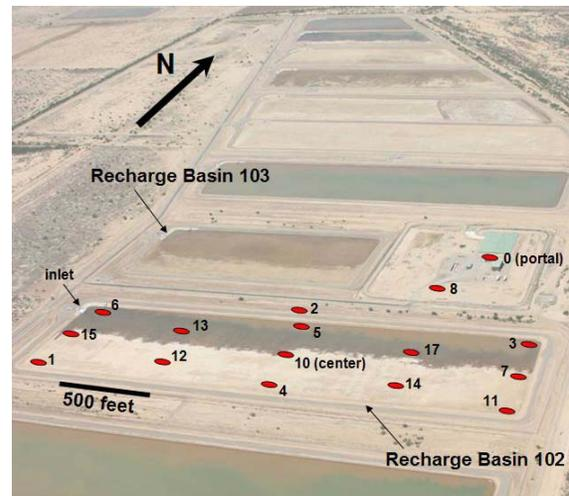
Figure 2: Oblique aerial photograph showing the location of the individual pods of the Sensor Web system at CAVSARP. The portal pod 0 is connected to a local server for Internet access.
