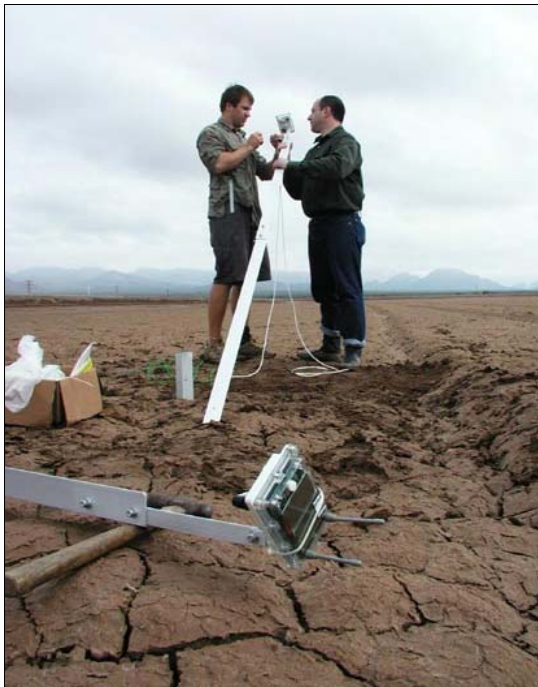
Figure 3: NASA/JPL team members deploy a Sensor Web pod in recharge basin 102. Extended stands allow the pods to stay operational (above water) during a basin flooding event.
