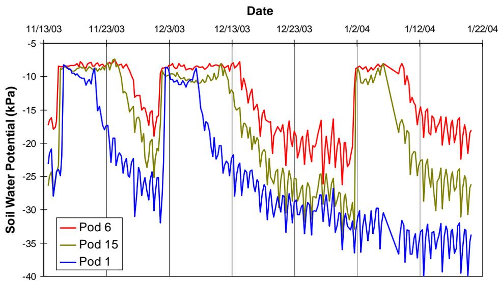
**Figure 9.** Soil water potential at 0.5 m deep along the west basin border. Note that the third flooding event did not last long enough to affect pod 1.
