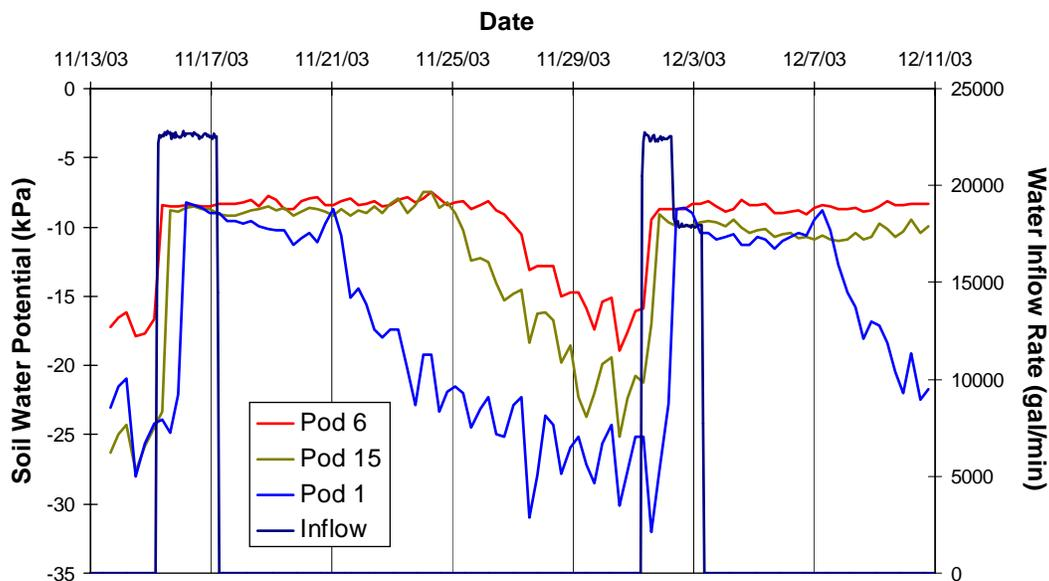
**Figure 8.** Soil water potential at 0.5 m deep along the west basin border during the first two flooding events after deployment. Traveling from north to south, the pods are positioned: 6 (inlet), 15, and then 1. Also shown is the inlet water rate.
