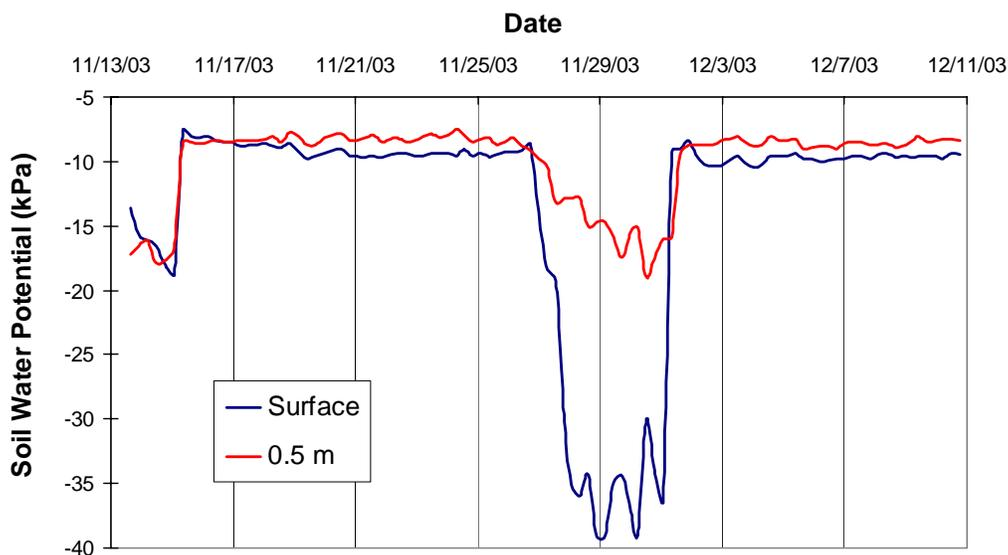
**Figure 10.** Comparison of pod 6 soil water potential at two depths.
