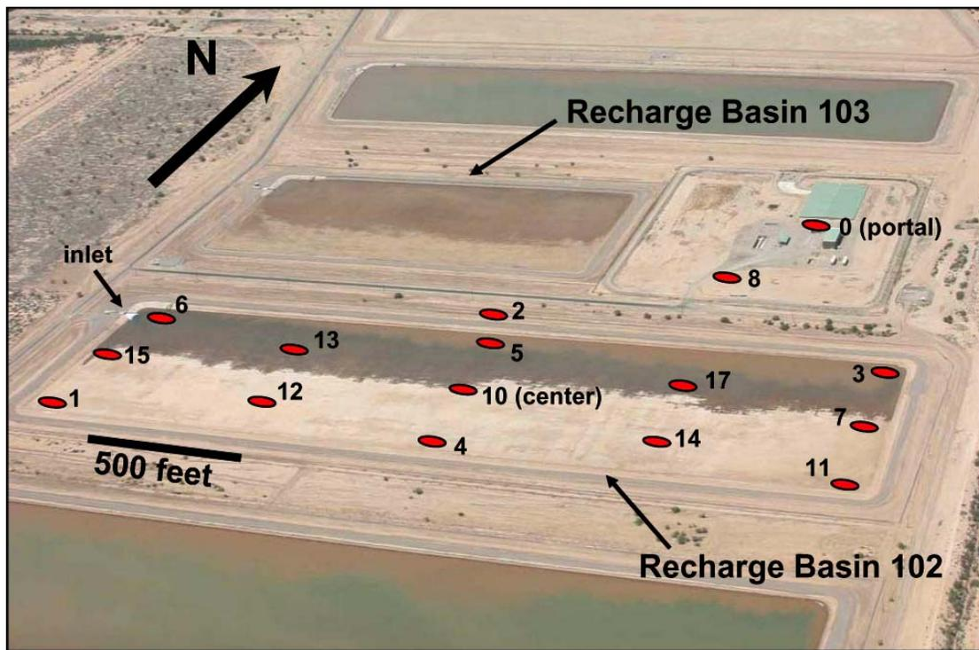
**Figure 4.** Aerial view of a portion of CAVSARP facility showing the location of the Sensor Web pods in recharge basin 102. The portal pod (pod 0) is connected to a computer which transfers the data to the Internet. In this photograph, recharge basin 103 is drying out, with the wetter soil in the northern portion of the basin. In contrast, basin 102 is being flooded with the moving water advancing southward. The basins immediately north of 103 and south of 102 are fully flooded.
