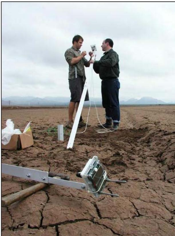
**Figure 5.** NASA/JPL team members deploy a Sensor Web 3.2 pod in recharge basin. Extended stands allow the pods to stay operational above water during a flooding event. Note polygon patterns in soil, indicative of previous flooding/drying cycles.
