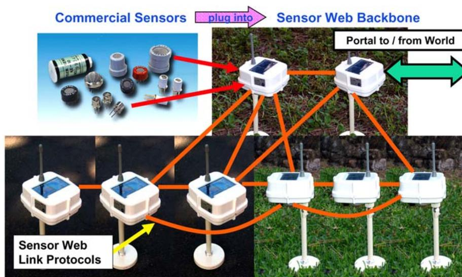
**Figure 2.** The Sensor Web forms an informational backbone that creates a dynamic infrastructure for the sensors in the Sensor Web pods.
